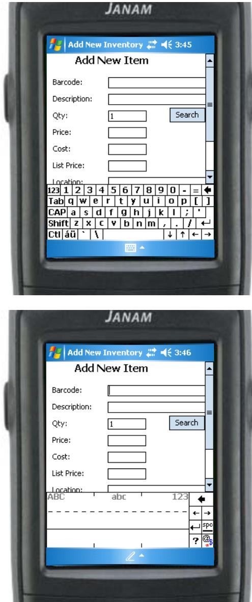
**Figure 117.** Software Keypads
